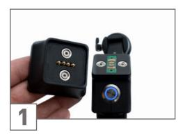
Remove the Protective Cap on top of the han- Attach the GPS Receiver by connecting it with dle of the Telescopic Rod.
