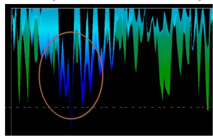
Example of a tunnel (single line): A scan may be repeated several times to ensure that the void is real and it does not move.
