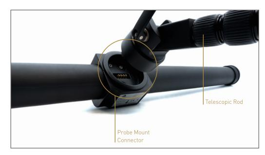
All measuring probes are equipped with a **Probe Mount Connector** that mounts the probe to the Telescopic Rod. To mount the probe, simply push it onto the probe mount of the Telescopic Rod. Thanks to the magnetic connection, the probe gets attracted in only one specific orientation to the probe mount connector.
