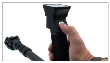
As soon as the Telescopic Rod is fully charged, remove the charger and push the Trigger Button at least 2 seconds until the LED ring of the Trigger Button lights up **green**. If the Control Unit is switched on as well, the Telescopic Rod will try to establish a wireless connection to it and – by success – the LED ring will turn **blue**.
