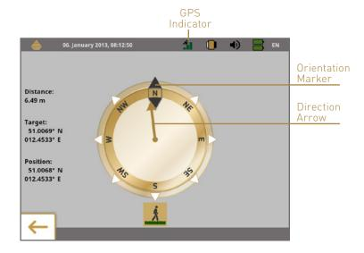
The **Position** indicates the GPS coordinates of your current position, while the **Target** is the place where you have performed your scan.
