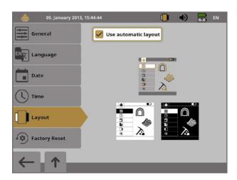
If you select the option "Use automatic layout", the eXp 6000 Control Unit selects the current layout automatically by measuring the light condition of the environment. If the light changes during operation the layout may change automatically.
