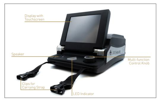
All functions are controlled by the **Multi-function Control Knob** or by using the touch capabilities of the display. To operate the device, rotate the knob to the desired function and push the knob to select it. Alternatively, simply tip with your finger onto an item on the screen.
