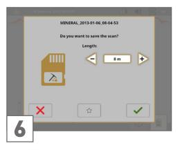
Click X to discard the current scan without saving or enter the correct scan line length and confirm with ✓ to save it.
