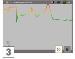
Walk a straight line. Don't change the height After finishing your scan, enter the scan line of the probe.
