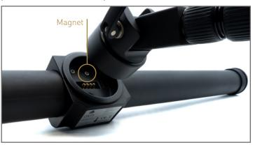
Please note: Each measuring probe can only be attached in one way or direction according to the magnetic connector of the probe mount.
