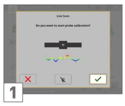
Hold your Live-Stream Sensor over neutral ground, which means normal underground without any potential objects.
