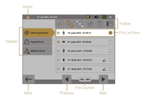
The **Sidebar** allows to switch between the operating modes.
