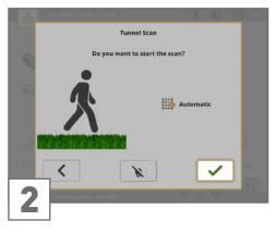
Go to your starting position and select ✓ to start the measurement. Start walking as soon as you press the Trigger Button because the eXp 6000 will record scan data immediately.
