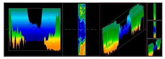
This scan was conducted using a normal 3D Ground Scan with multiple scan lines. When conducting a traditional ground scan, the parallel method of scanning must be used.
