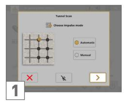
Select the operating mode Tunnel Scan and adjust the Impulse Mode.
