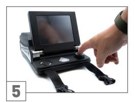
Push the Multi-function Control Knob at After a short moment the boot up screen will As soon as the home screen appears, you can Carry the eXp 6000 Control Unit around your least 2 seconds (until the LED Indicator stops appear on the display of the Control Unit. flashing and starts fading in various colors) to power on the detector.
