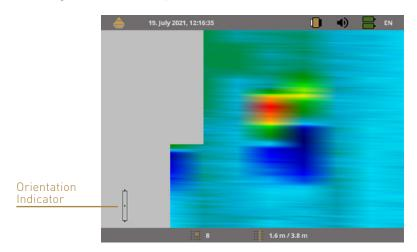
Please keep in mind that the **orientation indication** does not avoid rotational errors but informs you about the inclination of the probe in relation to the ground surface.
