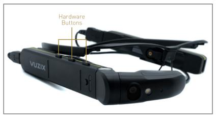
Use the **hardware buttons** to navigate through all menus and operating modes. Alternatively you may also use the Multi-function Control Knob of the eXp 6000 Control Unit to select any of the functions.
