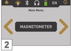
Power on the device and select "Magnetome- If a proper probe is connected, confirm the priate probe connected, the button is disabled button. and displays the 🚜 icon.
