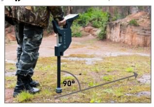
Move slowly forwards, backwards and sidewards, but avoid turning the probe. The probe should always point vertical to the ground. **DO NOT** pivot, swing or turn around its own axis.
