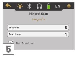
ready contains data from a previous scan, an confirmed to overwrite an occupied one, the Mineral Scan screen appears.
