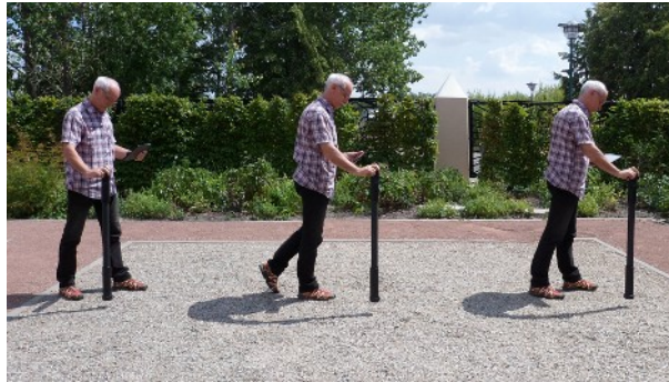
Figure 7.7: "Zig-Zag" scan in operating mode "3D Ground Scan"
